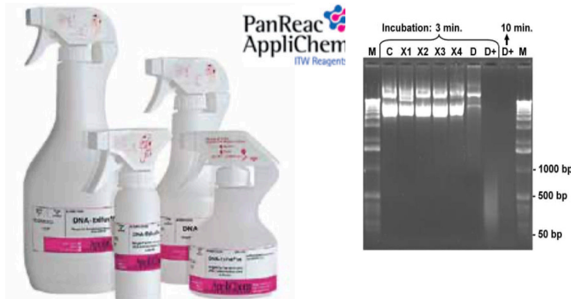
Fig. 1. Test of the DNA degradation potential for selected conventional DNA decontamination reagents in comparison with DNA-ExitusPlus™.
